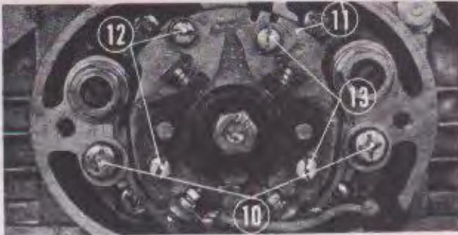
⑩ Base plate locking screws ⑪ Base plate
