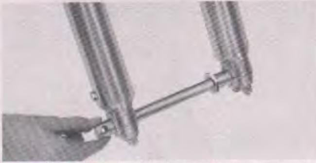
Fig. 8-10. Aligning both front axle holes
