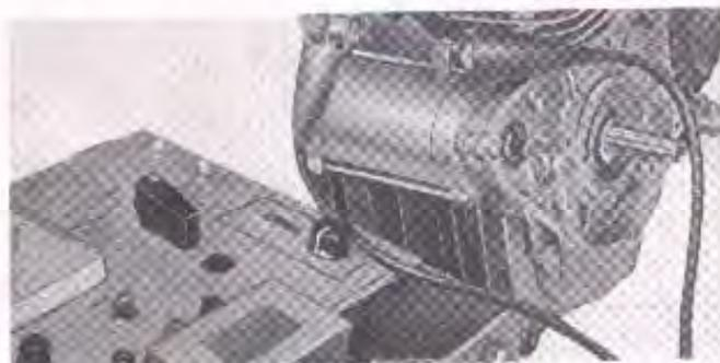
Fig. 6-55. Starting motor current measurement
