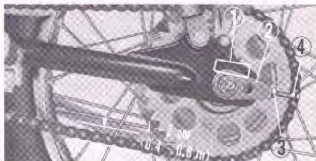
① Reference mark ② Drive chain adjuster ③ Lock nut
