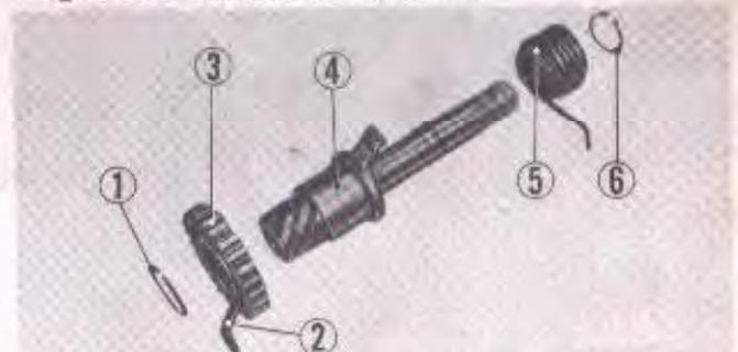
① 25 mm circlip ② Friction spring
