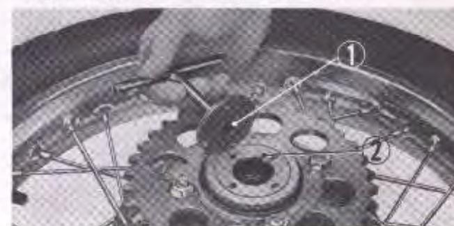
① Bearing retainer tightening wrench
