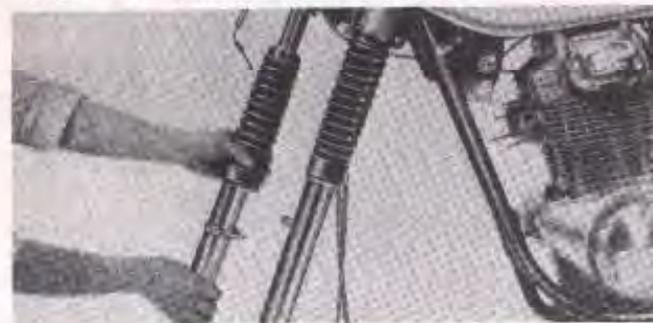
Fig. 5-27. Installing the front fork into the steering
