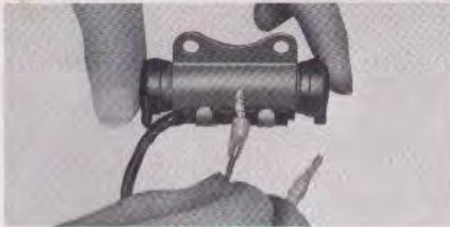
Fig. 6-20. Short-circuiting of the condenser
