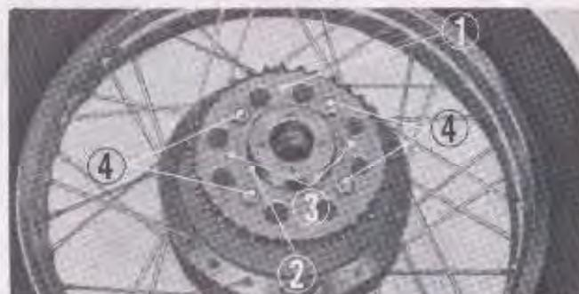
① Final driven sprocket ② 69 mm external circlip
