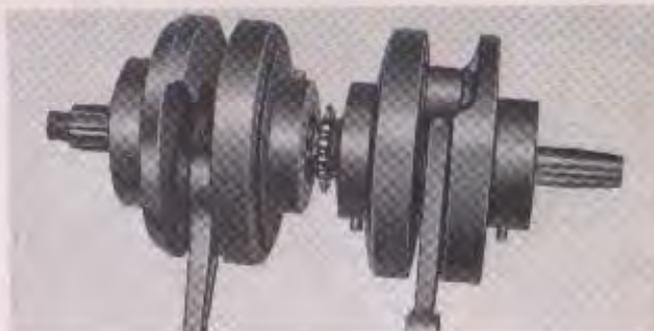
Fig. 4-90. Crankshaft
