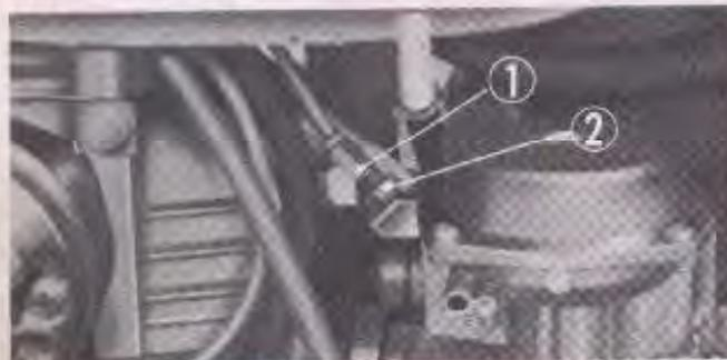
① Throttle cable adjust bolt ② Lock nut
