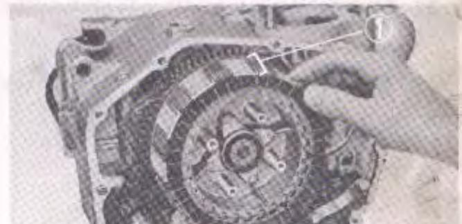
① Clutch plate and friction disks
