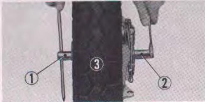
① Front wheel axle ② Front wheel axle sleeve
