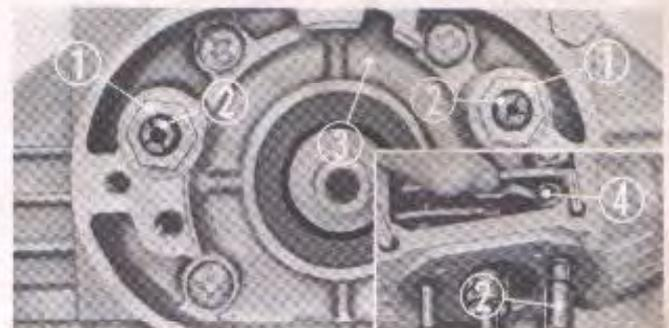
① Rocker arm pin lock nuts ② Rocker arm pins
