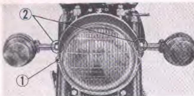
① Adjusting screw ② Headlight mounting bolt
