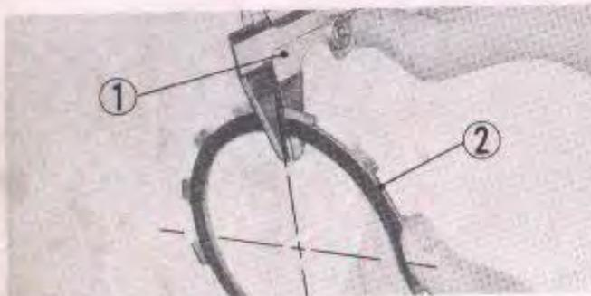
① Vernier caliper ② Friction disk
